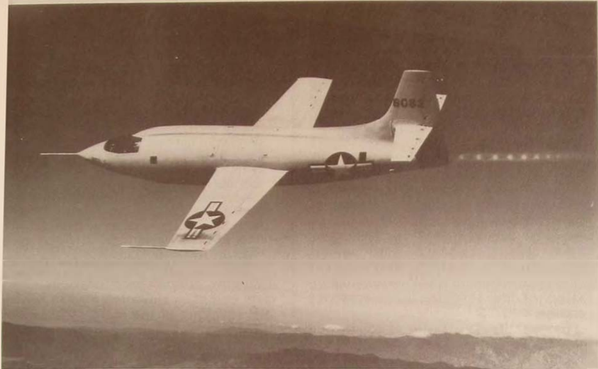
The Bell X-1 (formerly the XS-1) was a rocket-powered experimental plane built for transonic flight. Piloted by Capt Charles Yeager, it made its first supersonic flight on 14 October 1947.
